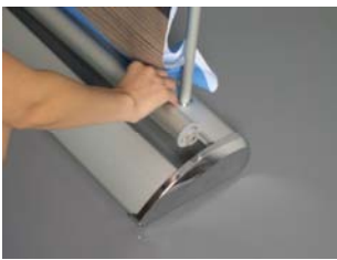
Step 7: Take out the bottom graphic roller from the base.
