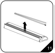
10. Open the front cover and remove the telescopic pole from the storage compartment. Close the front cover.
