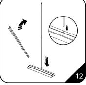
11. Unfold the telescopic pole and insert the round end into corresponding hole in the base.
