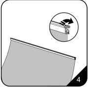
4. Close the top snap rail fully to secure the graphic. It may be easier to lay the graphic on a table and push down hard to close the snap rail completely.
