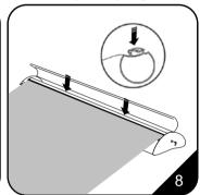
8. Close the roller's snap rail by pushing down firmly on the rail to secure the banner.
