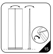
14. The unit can be leveled by adjusting the threaded plastic feet at the bottom of the base unit.
