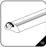
10. If there is not sufficient tension on the roller to fully retract the banner, turn the tension knob on the left end of the base clockwise until the banner is fully retracted, then turn an additional 4 revolutions.
