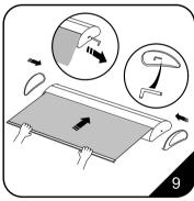
9. Remove the locking pin from the right side end plate while holding the banner securely. Let the banner slowly retract into the base. Store the locking pin and replace the end caps removed in Step 6.
