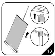
13. Grasp the top rail of the banner and attach it to the plastic holder at the top of the pole. An arrow indicates the spot where the pole should be inserted.
