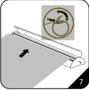
7. Open the roller's snap rail by lifting up the back edge of the rail, insert the bottom edge of the banner into the opening with the back of the graphic facing up.
