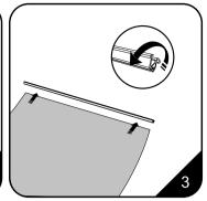
3. Open the top snap rail then insert the top edge of the graphic as far as it will go.
