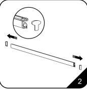
2. Remove the plastic end caps from the top snap rail.
